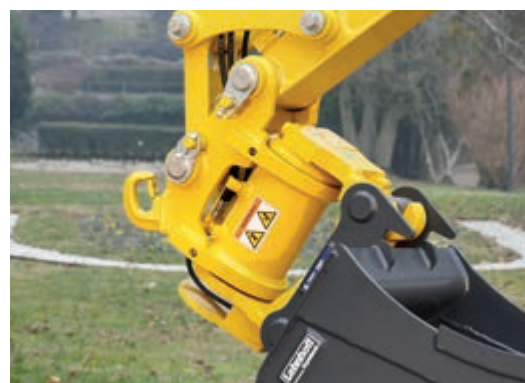
Lehnhoff Powertilt is available as factory fit. It combines all benefits of a quick-coupler with a tilt motor, offering a huge work range of 2 x 90° swivel range to both sides.
