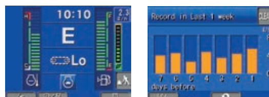
Updated monitoring system, including Eco-gauge and fuel consumption gauge, as well as extended maintenance and operational data reports.
